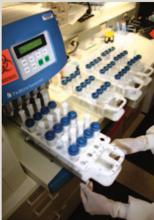
A technologist processes specimens for liquid-based Pap smears by using the BD PrepStain™ Slide Processor, which prepares up to 40 slides at one time. The group processes up to 48 slides a day.
