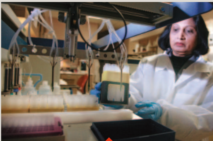
Shobha Patel, laboratory manager in the Section of Cytopathology, loads the BD PrepStain™ Slide Processor, which prepares and stains slides so Pap smears can be evaluated.
